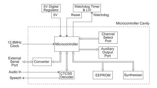
Figure 2.5 T825 Microcontroller Block Diagram
