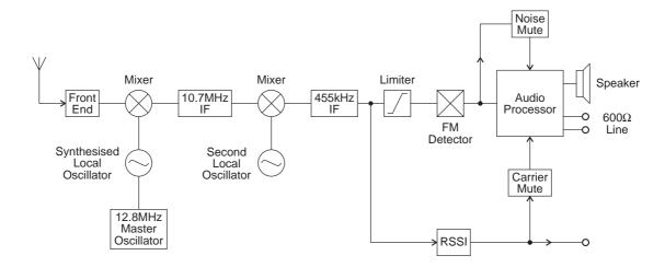
Figure 2.1 T825 High Level Block Diagram
