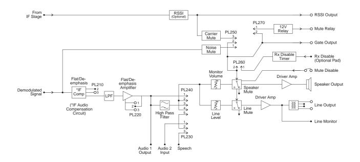
Figure 2.3 T825 Audio Processor Block Diagram
