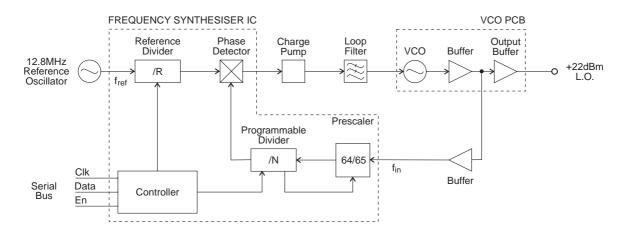
Figure 2.6 T825 Synthesiser Block Diagram
