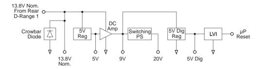
Figure 2.4 T825 Power Supply And Regulators Block Diagram
